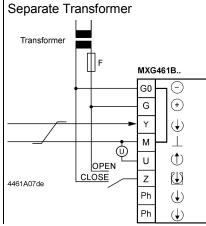
**Terminal assignment** for controller with 3-wire connection DC 0...10 V DC 2...10 V
