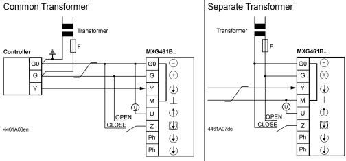
Indication of valve position (only if required). DC 0  $\stackrel{'}{...}$ 10 V  $\rightarrow$  0...100 % volumetric flow V<sub>100</sub>
